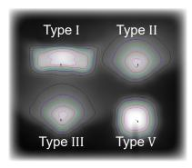
Each lamp is supplied in one of four different lighting distributions: (Type I, II, III, or V).
